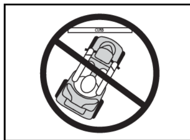
Figure 11.b Incorrect Curb Approach
